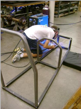
Sean welding the chassis
