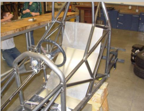
We are fitting the seat, and installing the steering. We recently finished constructing the back end.
